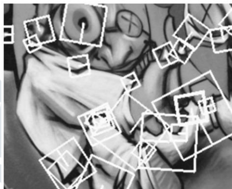
Fig. 9: Detail of the Graffiti scene showing the size of the oriented descriptor window at different scales.
