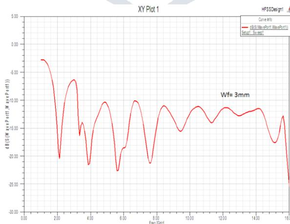
Figure 5.2  $s_{11}$  for  $W_f=3\text{mm}$
