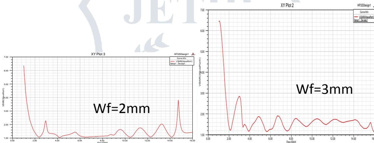
Figure 6.1 VSWR for Wf=2mm
