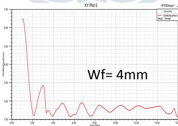
Figure 6.3 VSWR for Wf=4mm
