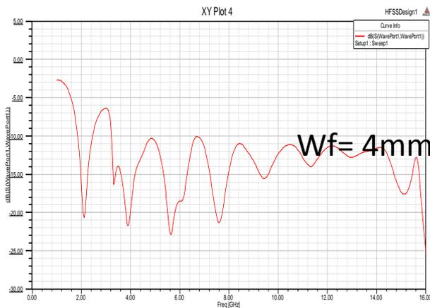
Figure 5.3 s11 for Wf=4mm
