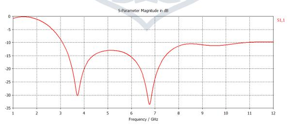
Figure 2 S<sub>11</sub> vs Frequency graph RETURN LOSS S<sub>11</sub> RESULT
