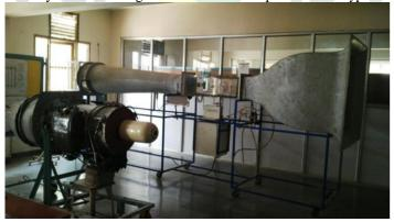
Fig. 5.1: Wind tunnel
