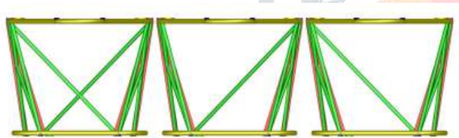
Fig. 16 From left to right, cross brace, “/” brace, and “\” brace, each inserted to lower driver cockpit in alternating sequence
