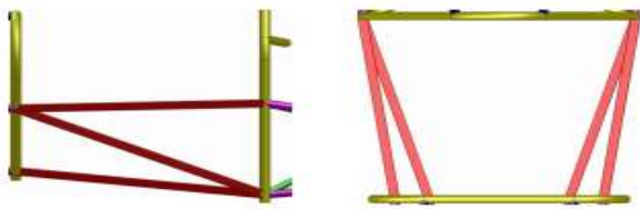
Fig. 14 From left to right, side driver cockpit (side view) and lower driver cockpit (plan view)
