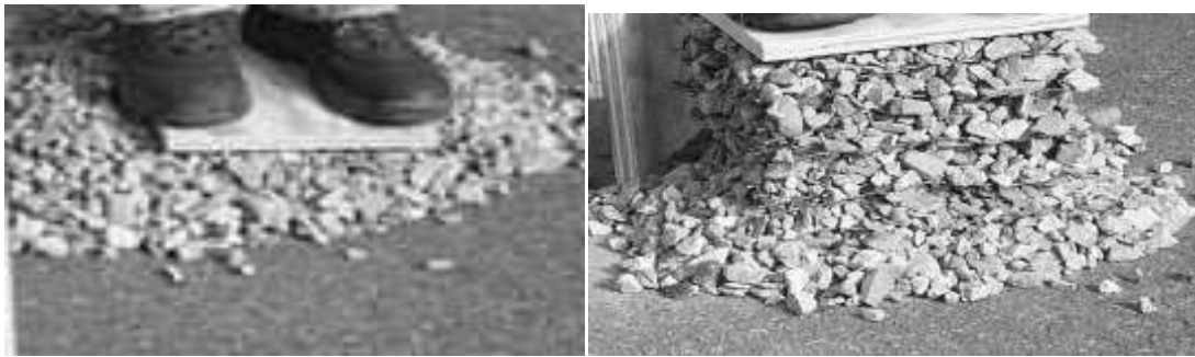
Fig 13 Aggregates compacted without geogrid layers Fig 14 Aggregates compacted with geogrid inceted in layers
