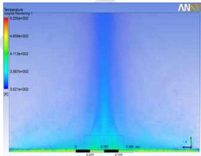
Fig.8 volume rendering of temperature perforated fin array(s=2)
