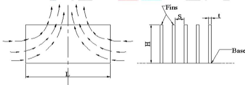
Fig.2 single chimney flow pattern
