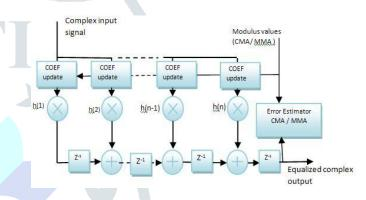
Fig. 3 High Level CMA / MMA Blind Equalizer
