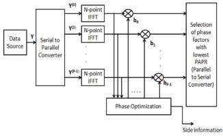
Fig. 2: Partial Transmit Sequence Method
