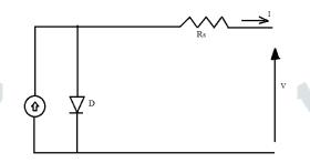
Fig 2: Solar cell model using single diode
