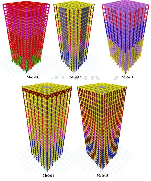
Fig,1 All Structural System ETABS 2015 Model
