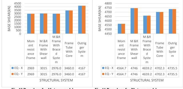
Fig. 10 Base shear for 10 storey model
