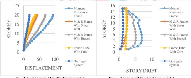
Fig. 4 displacement for 20 storey model
