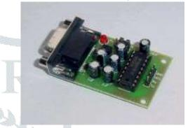
Work with 5V and 3.3V Power. The 3 pin jumper selects power from the PC or an external power source. Dimensions: 32 mm x 50 mm JUMPER information: POSITION 2-3: board will use power from PC serial port +5V. POSITION 1-2: board will use External Power +3.3V or +5V.
