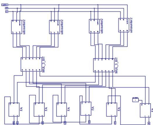
Fig 4- Direct digital synthesizer
