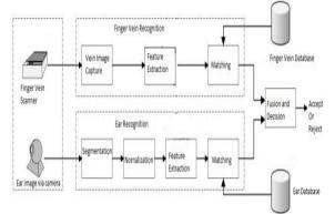
Fig.3. Architecture for fusion of ear and finger vein biometric
