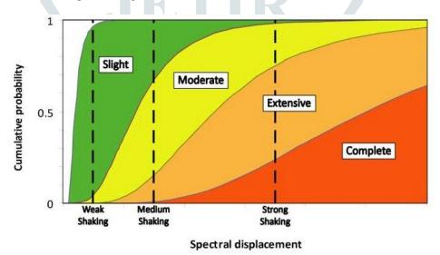
Figure 3: Fragility curves for 4 different limit states (Tobas and Lobo 2008)
