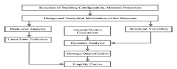
Figure 1 the methodology used in the derivation of fragility curves
