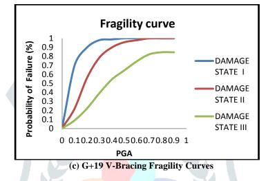
Graph 3: Fragility Curves of G+19 for (a) Bare (b) X-bracing (c) V-bracing
