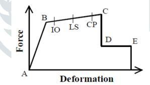
Figure 4: Force-Deformation for Pushover Hinge (Habibullah.et al., 1998)
