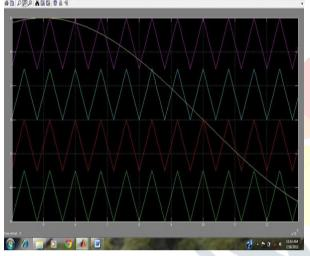
Fig.2 Triangular Waveform Simulation of Five Level Diode Clamped Inverter (PD PWM Technique)
