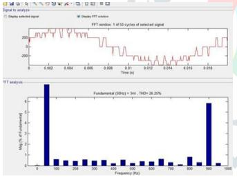
Fig.12 Harmonic Spectrum of Five level diode clamped Inverter Phase Voltage at modulation Index=1 (APOD PWM Technique).
