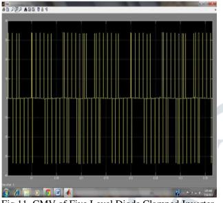
Fig.11 CMV of Five Level Diode Clamped Inverter (APOD PWM Technique)
