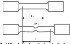
Fig. 4.3 Recycle Aluminium Specimen for Tensile test
