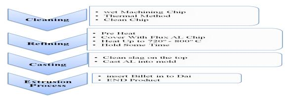
Fig. 4.1 Flow chart of recycling process of Al through hotbackward Extrusion
