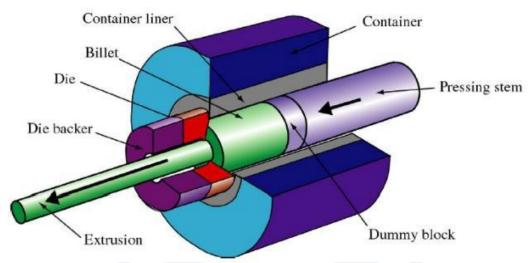
Fig.1.4. Illustration of extrusion process by Kalpakjian,S.
