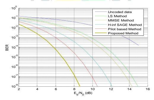
FIG 8: PLOT OF BER V/S EB/NO(DB) OF THE CONVENTIONAL AND PROPOSED METHOD FOR BPSK MODULATION SCHEME
