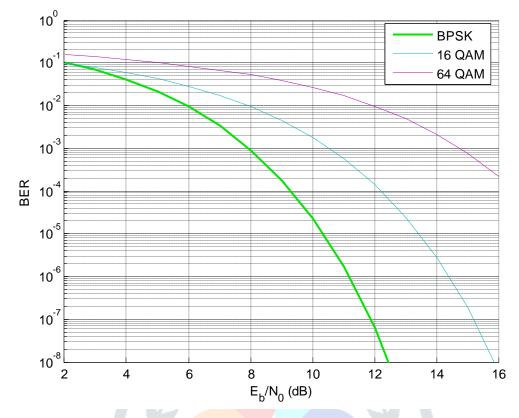
FIG 7: PLOT OF BER V/S EB/NO. FOR DIFFERENT MODULATION TECHNIQUE
