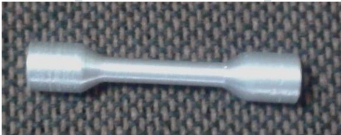
Figure 1: Photograph showing the tensile specimen
