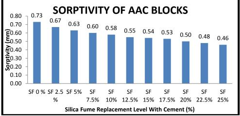
Fig. 1.5(e) Sorptivity of AAC blocks
