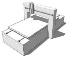
Figure 3 Moving Table Router
