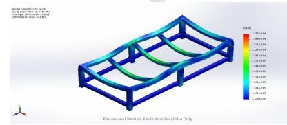
Figure 12 Equivalent Stress analysis of NR-115 Base Structure
