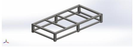
Figure 6 Geometry of NR-115 Base Structure using static analysis
