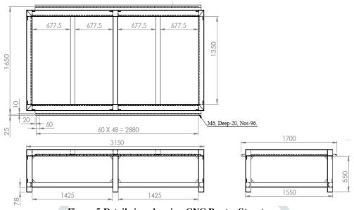
Figure 5 Detail view drawing CNC Router Structure
