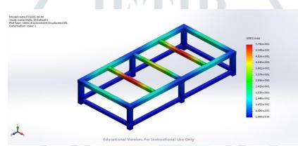
Figure 11 Dis placement of NR-115 Base Structure
