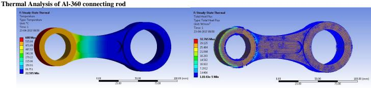
Fig23: Temperature Distribution
