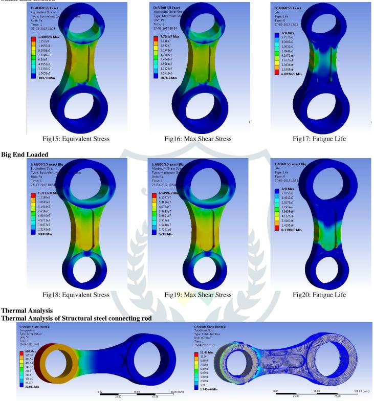
Fig21: Temperature Distribution
