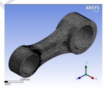
Fig 5: Details of Mesh
