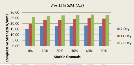
Figure 3: Comp. Strength of Mortar For 1:3 Proportion After Replacement Of 15% SBA
