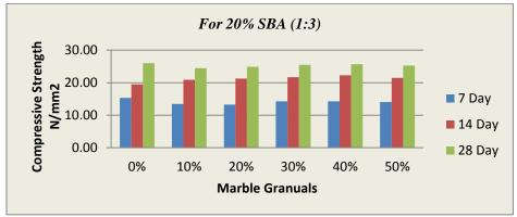
Figure 4: Comp. Strength of Mortar For1:3 Proportion After Replacement Of 20% SBA Journal of Emerging Technologies and Innovative Research (JETIR) www.jetir.org
