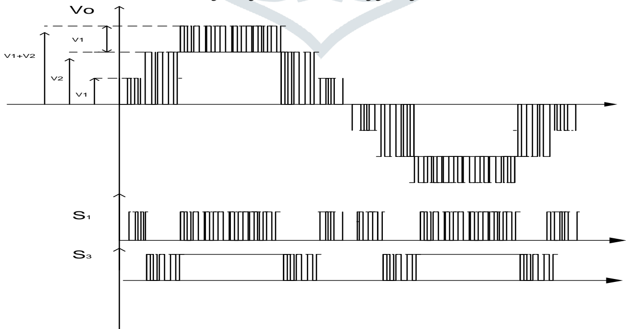
Fig. 8 Output of seven level asymmetrical inverter with proposed PWM operation.
