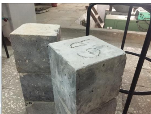
Figure 4 Salt Ponding Test
