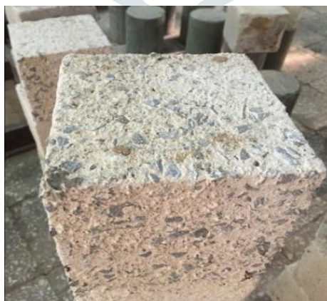
Figure 5 Acid Ponding Test
