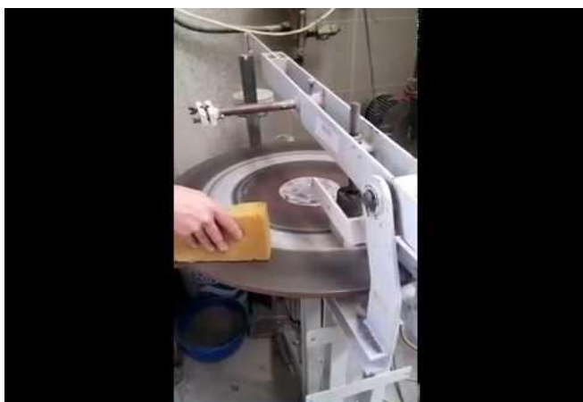
Figure 8. Abrasion Resistance (Bohme test)
