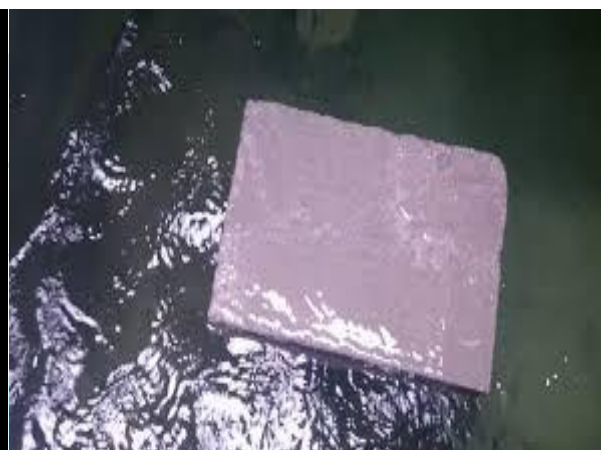
Figure 9. Water absorption test for paver block
