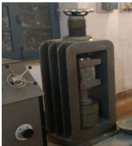
Figure 1 Test set up for compressive strength on cube fly ash concrete specimen
