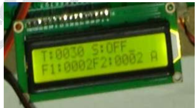
Fig 4: Monitoring the sensor values and Floor 1 & 2 count is started
