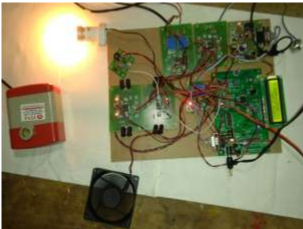
Fig 6: Appliances Motor, Bulb, Fan is Activated after the count increased in both floors
