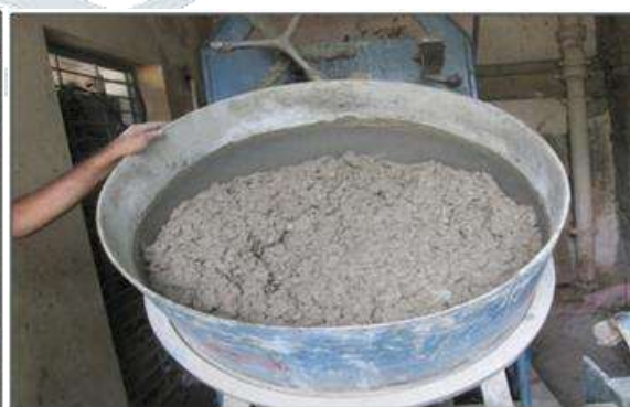
Figure 2 View of Fresh GPC Mixture
