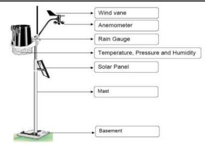
Fig.2: Schematic of the Automatic Weather Station installed at Inagalur, Kadapa District and Mypad, Nellore district.
