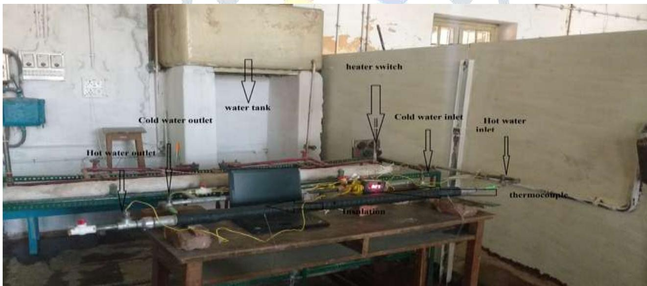
Figure. 3 Experimental setup of heat exchanger
