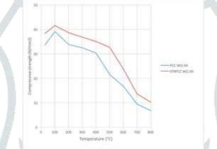
Fig 5: Variation of compressive strength with temperature for water quenched cube specimens exposed for 3 hours
