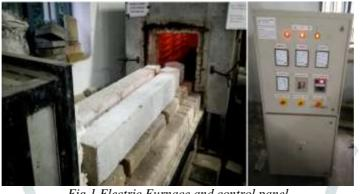
Fig 1 Electric Furnace and control panel
