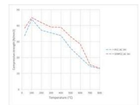
Fig 4: Variation of compressive strength with temperature for air cooled cube specimens exposed for 3 hours
