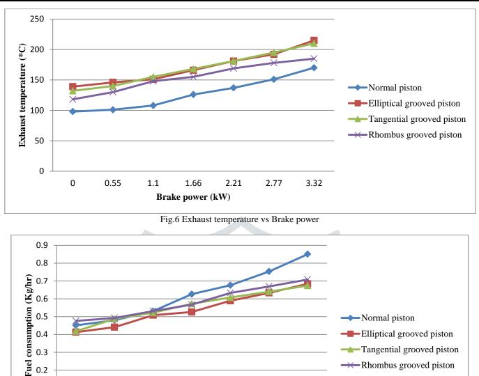
power. The specific fuel consumption of TGP less as compare to other groove pistons. From the Fig.5, it is absorber that the Brake thermal efficiency of grooves pistons are more as compare to normal piston by increase brake power. The Brake thermal efficiency of EGP more as compare to other groove pistons.
