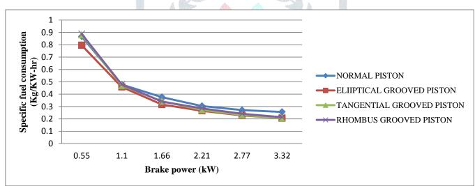
Fig.4 Specific fuel consumption vs Brake power
