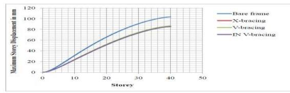
Figure 4: Maximum Storey Displacement in X- direction with X, V and inverted V bracing type. (When single bay is braced).
