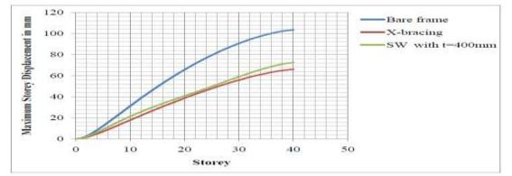
Figure 8: Double bay bracing Storey displacement in X- direction for 400 mm shear walled frame and X- braced frame. (When a double bay is braced and shear walled).
