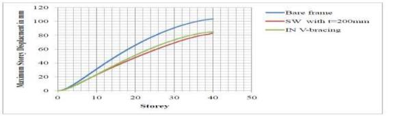
Figure 5: Maximum Storey displacement in X- direction for 200 mm shear walled frame and inverted V- braced frame. (When single bay is braced and shear walled).
