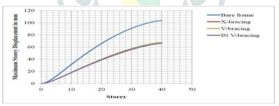
Figure 6: Double bay bracing Storey Displacement in X- direction with X, V and inverted V bracing type (When a double bay is braced).
