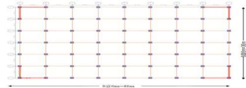
Figure 1: location of bracings and shear wall, when provided in a single bay
