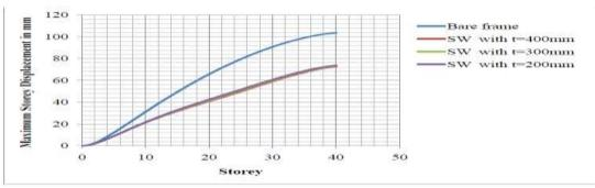
Figure 7: Double bay bracing Storey Displacement in X- direction with 200,300, and 400 mm thickness shear walled frame with reference to bare frame. (When a double bay is shear walled).
