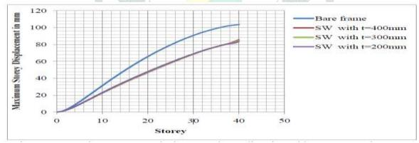
Figure 3: Maximum Storey Displacement in X- direction with 200,300, and 400 mm thickness shear walled frame with reference to bare frame. (When single bay is shear walled).
