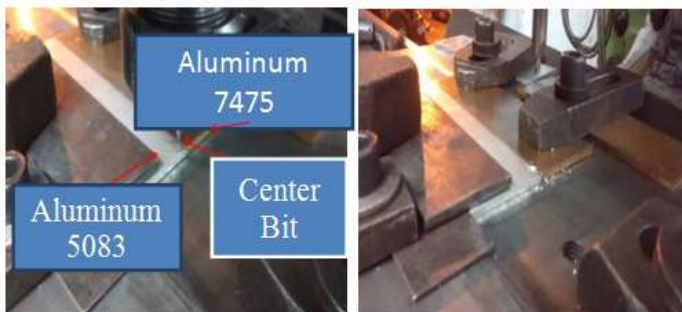
Creation of plunge depth by using a center bit
