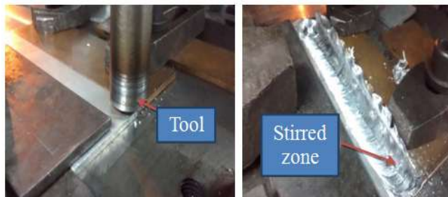
Creation of plunge depth by using a center bit
