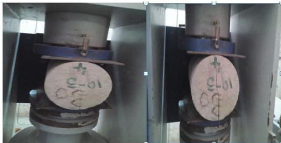
Fig: Testing the specimen in split tensile strength
