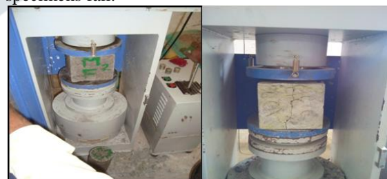
Fig: Test of specimens for compressive strength
