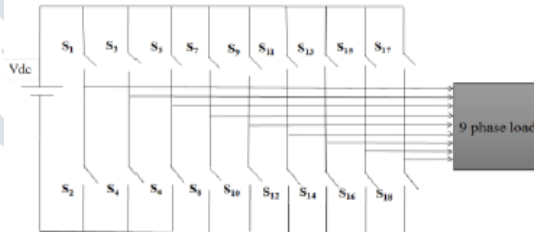
Figure.4. Topology of Nine Phase Inverter
