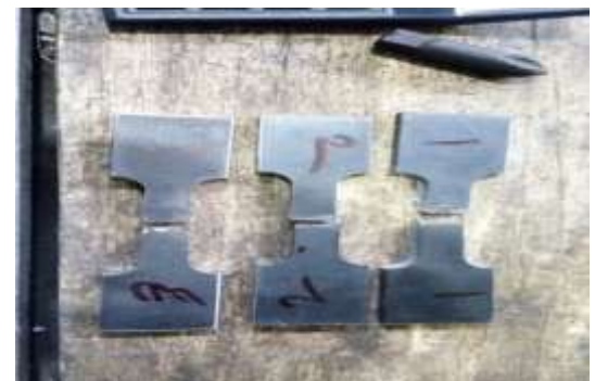
Dumbbell shape work pieces for tensile test Work pieces setup
