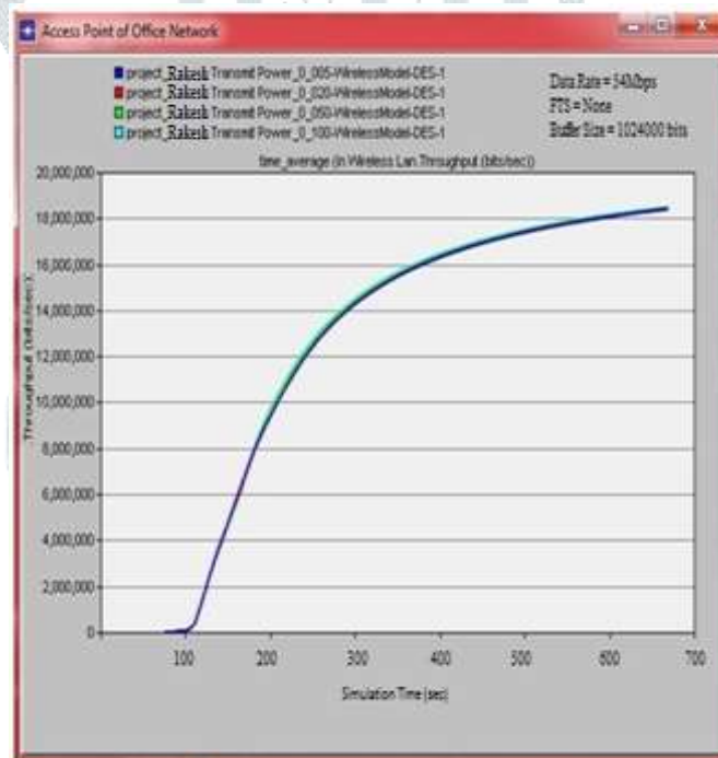
Fig.9 Throughput results for different transmit power
