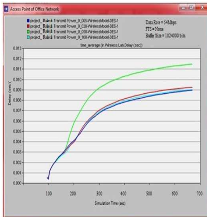
Fig. 6 Delay results for different transmit power
