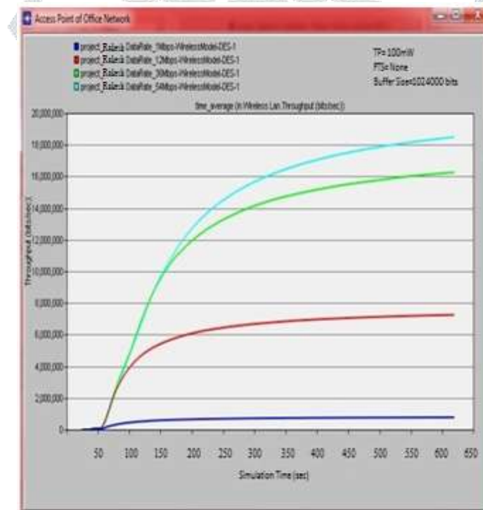
Fig. 5 Throughput Study for data rates 1Mbps, 12Mbps, 36Mbps and 54Mbps
