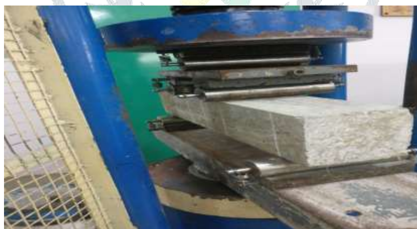
Fig. 4.3 Flexural Test On Beam
