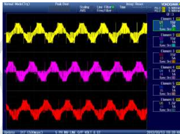
Fig.8 Line to line voltage from the inverter
