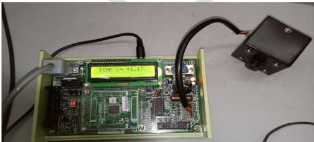
Fig.31 Rise in temperature value displayed on the LCD
