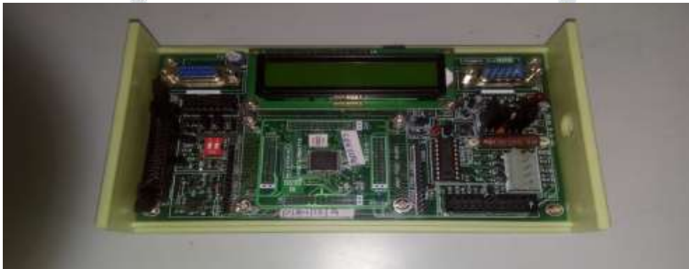
Fig.1 Photographic view of the ARM-09 NXP LPC2148 Microcontroller Board
