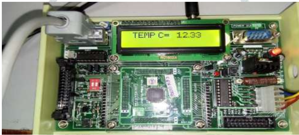
Fig.30 Reduced temperature value displayed on the LCD
