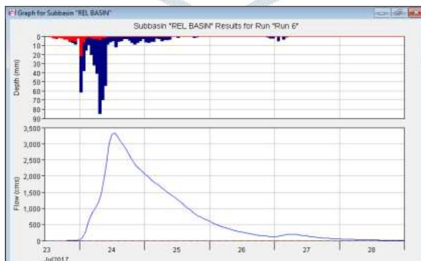
Figure 5 Outflow Hydrograph of Calibration
