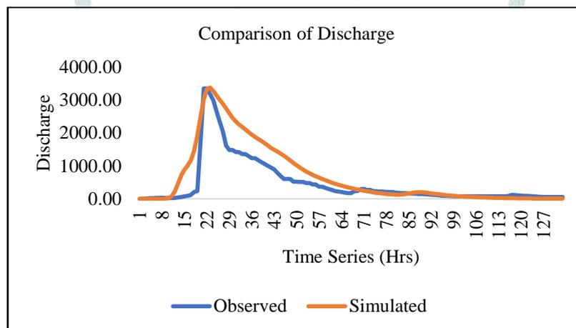
Figure 6 Comparison of Simulated and Observed Discharge for Validation
