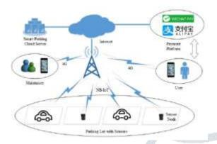
It comprises of sensor node (Geo-magnetic vehicle detector), cloud server, mobile application and a third-party payment platform. Sensor node is installed in the parking area and continuously detects the changes if any changes occur then it updates on the server and user can pay the parking charges online[10].
