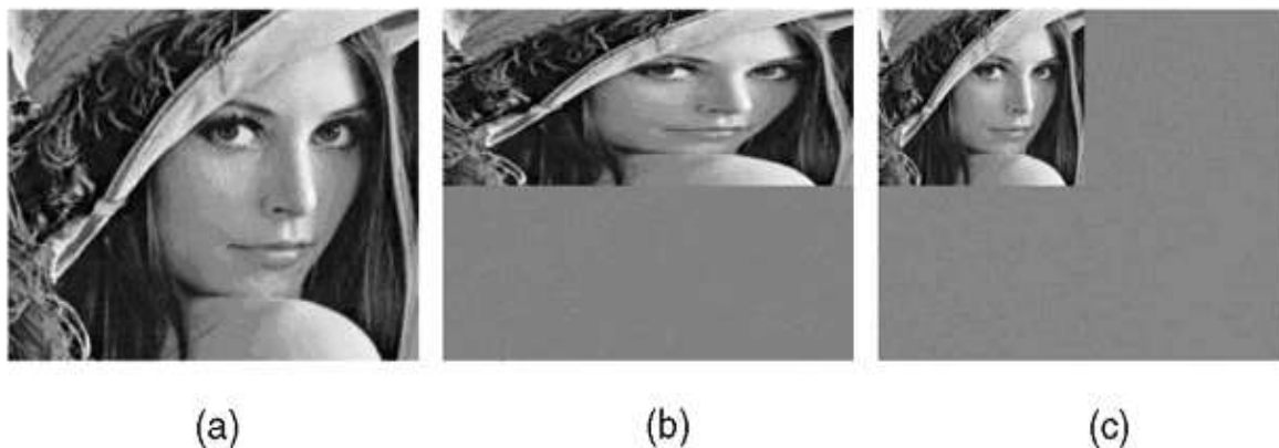
Fig 7: DWT for Lena image (a) Original Image (b) Output image after the 1-D applied on column input (c) Output image after the second 1-D applied on row input
