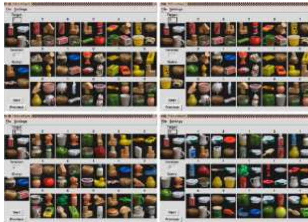
Fig. 10. Result of relevancy feedback learning for a database containing mixed objects of varying textures and color. The progression of images is from top left to bottom right. The desired target image is shown on the top left of each screen shot and the query image is shown on the bottom left. The numbers above each retrieved image correspond to the relevancy ranking assigned by the user. It corresponds to the number of object in the image that are of interest to the users. The images is taken from [30].
