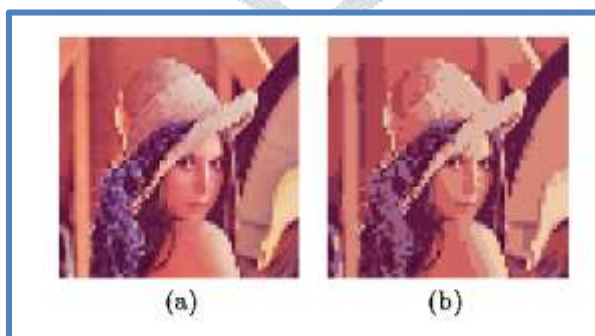
Fig. 7. Results of segmenting a 64x64 color image using DeMenthon’s et al. Hidden Markov mesh model. The original image (a) has been segmented in ten regions (b). From [23].
