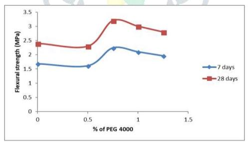
Figure 6. Variation of Flexural Strength with varying %age of PEG-4000 for 7 and 28 days.
