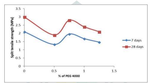
Figure 5. Variation of Split Tensile Strength with varying % age of PEG-4000 for 7 and 28 days.
