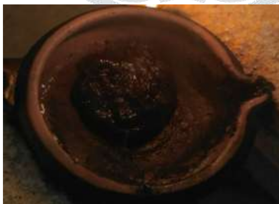
Figure 3: Semi solid polyethylene after melting of polyethylene bags in a graphite crucible.
