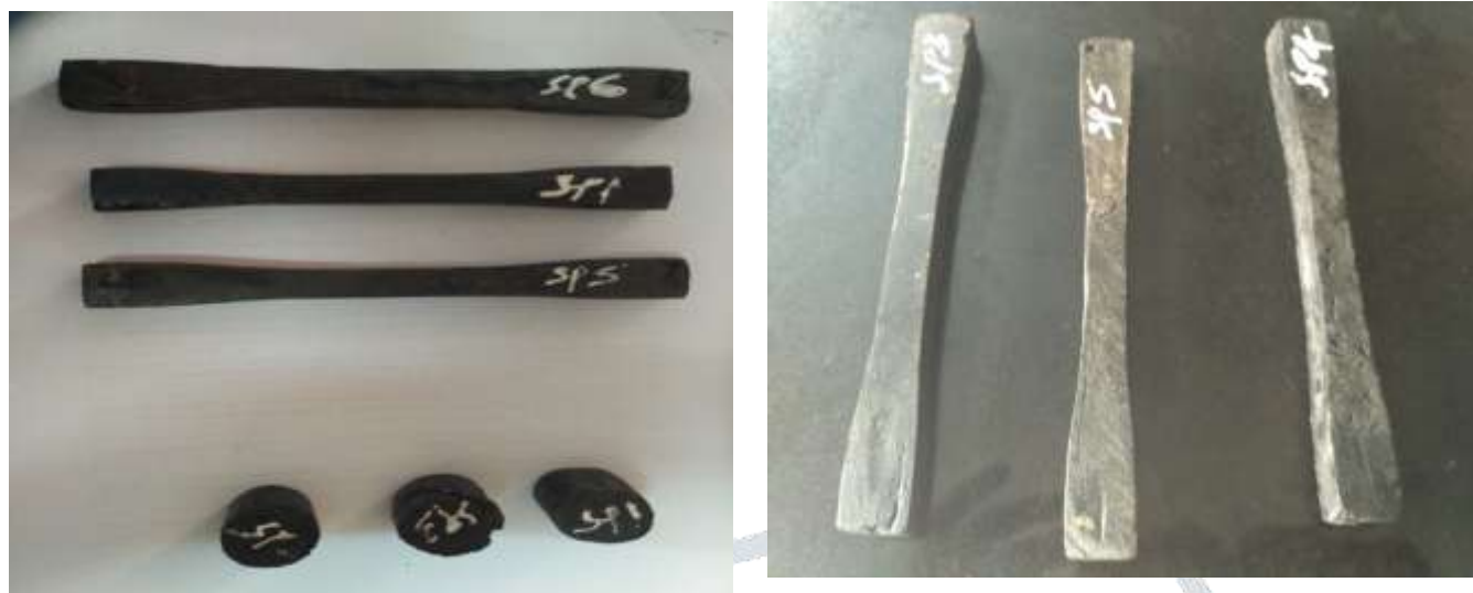
Figure 7: Prepared tensile and compression test specimens made of LDPE.
