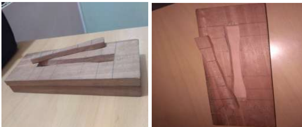
Figure 1: Mould for tensile testing specimens.
