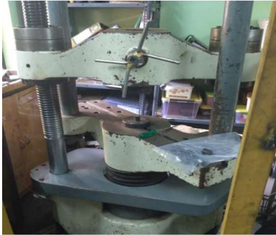
Figure 9: Universal testing machine used for testing of wood plastic composites.
