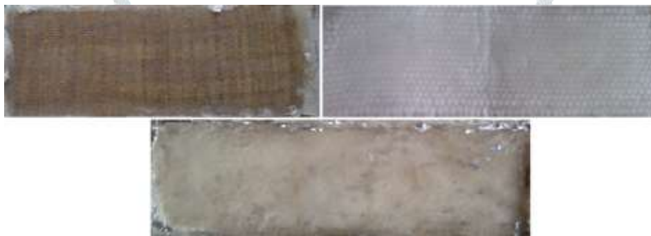
Fig3.6. Fabricated composites of nettle fiber, woven glass fiber, random glass fiber, clockwise from the top.
