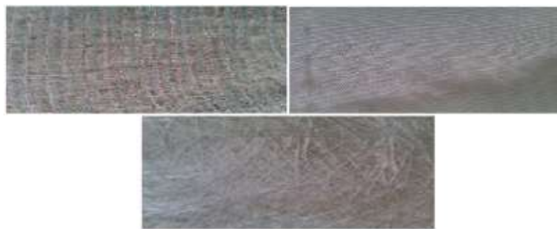
Fig 3.4 Fibers clockwise from top-left nettle fiber, woven glass fiber, random glass fiber.
