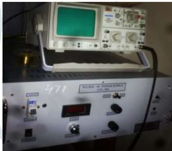
Figure 8: Photograph of pulsed DC Power Source
