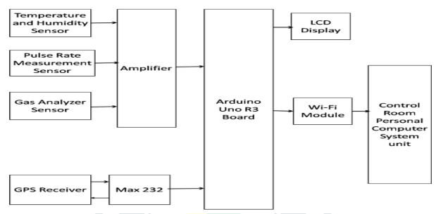
Figure 1 Constructional block diagram of IoT based soldier position tracking and health monitoring system
